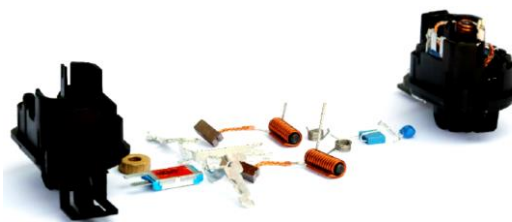
Fig. 2. Components of micro-motor flanges [17]
