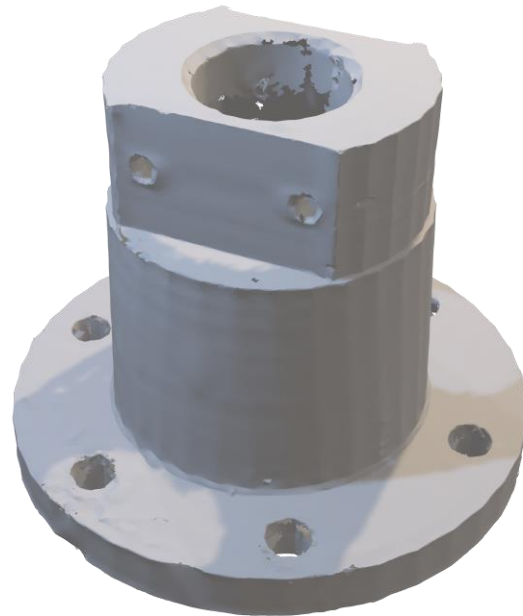
Fig. 8. Scanned model of the "Coupling flange" part
