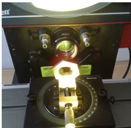
Fig. 1. Attach the part to the measuring device
