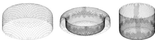
Fig. 10. Deformation stages in reverse redrawing
