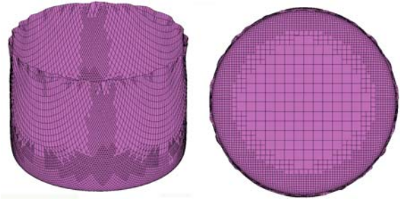
Fig. 15. Form variation in reverse redrawing
