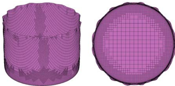
Fig. 14. Form variation in direct redrawing
