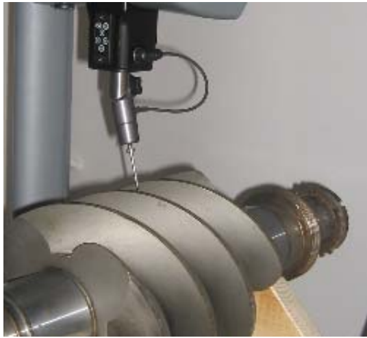
Fig. 2. Male rotor on the machine Micro Hite 3D
