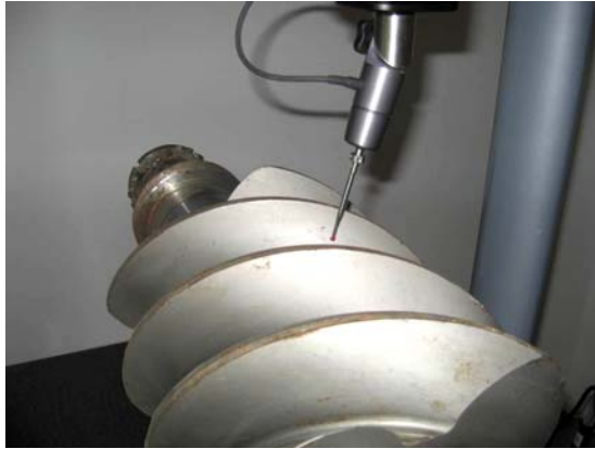
Fig. 2. The measuring of the rotor's axial profile
