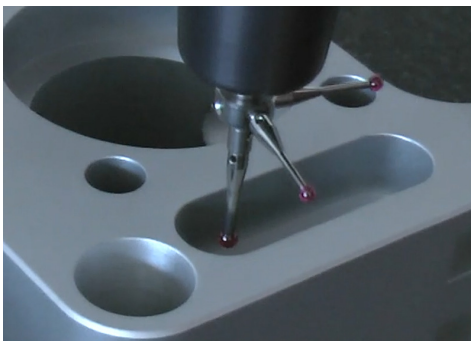
Fig. 1. Probes in the 3D measurement machine
