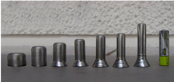
Fig. 9 Deep-drawn cups of high strength steel sheet (980 MPa TS) (Aida Engineering Ltd.)
