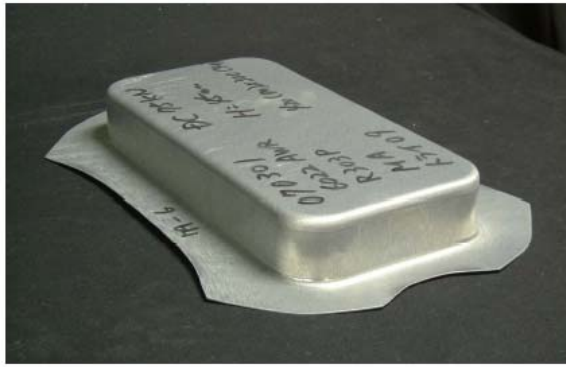
(b) Panel formed at high velocity (103mm/s)
