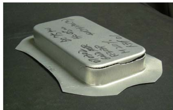
(a) Panel formed at low velocity (41mm/s)
