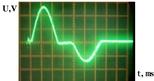
Fig. 4. General view of the oscillating graph obtained by means of the source described above in the discharge circuit: U_c=400\text{ V} , S=1,5\text{ mm} , C=8\ \mu\text{F} , f=8\text{ Hz} .
